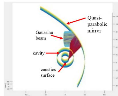
**Figure 3** Schematic diagram of the quasi-parabolic mirror with optical path
