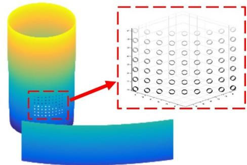
**Figure 2** TE<sub>28,8</sub> mode generator and grid of the coupling holes in the cavity wall
