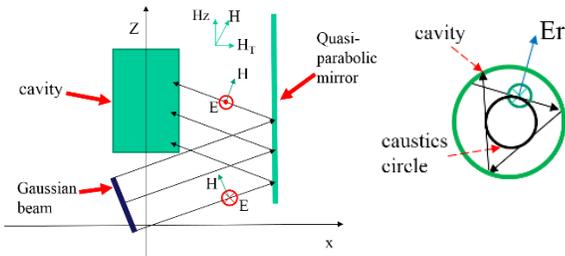
**Figure 4** Polarization of the Input Beam Field
