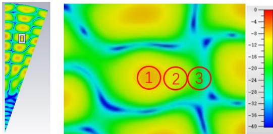
**Fig.5**  $TE_{28,8}$  electric field distribution in an azimuthal direction period and the positions of three detected points
