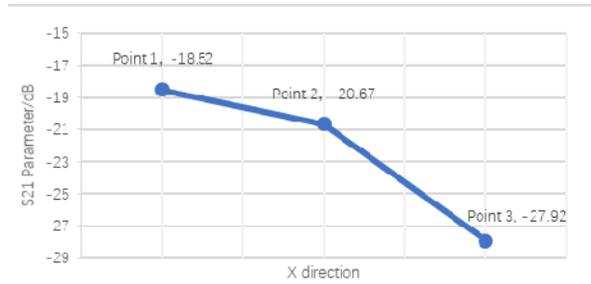
**Fig.6**  $S_{21}$  Parametric curves at three points
