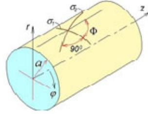
Figure 2. Sheath helix with finite values of conductivities.
