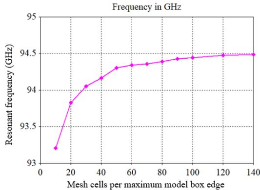
**Figure 3.** Resonant frequency of the ARMRC vs. number of mesh cells per maximum model box edge ( $2\pi$ -mode).
