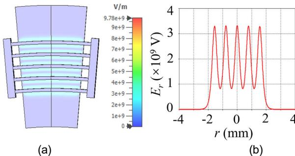
**Figure 4.** (a) Electric field distribution and (b) radial electric field of the ARMRC ( $2\pi$ -mode, 94.5 GHz).
