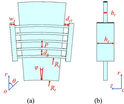
**Figure 2.** Structure parameters of the proposed ARMRC on (a)  $r\theta$  plane and (b)  $rz$  plane.
