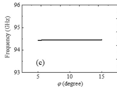
**Figure 5.** Resonant frequencies of the  $2\pi$  mode with different (a)  $R_c$ , (b)  $h_c$  and (c)  $\varphi$ .
