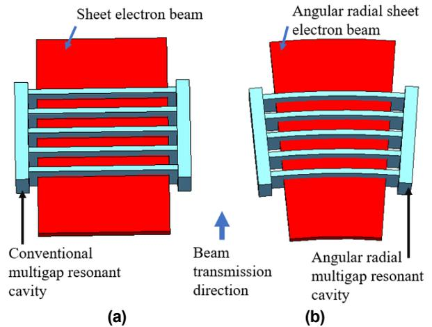
**Figure 1.** Comparison between the 3D models of (a) conventional sheet beam five-gap resonant cavity and (b) proposed ARMRC.
