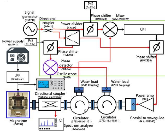
**Fig. 3.** Experimental configuration for injection locking with the phase locking loop (PLL). PLL mainly consists of a double balanced mixer detecting the phase difference between the reference and the magnetron and a control circuit (CKT) producing the voltage to adjust the phase of the phase shifter.
