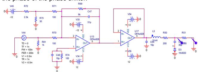
**Fig. 4.** The schematic diagram of the CKT. The voltage to adjust the phase is produced by the inversion amplifier and offset bias, then applied to the phase shifter through the buffer. The operational amplifiers employed in the PLL has 150V/μs of slew rate and 45 MHz of open gain bandwidth. Resistances and capacitances were determined considering the circuit response and optimized by PSpice simulation.
