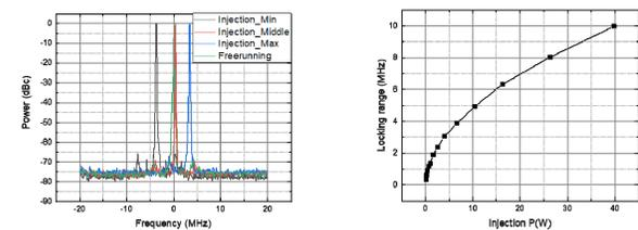
**Fig. 2.** Left: Example of frequency control by injection. Right: Frequency locking range with respect to the injection power at the operation of 80% of the maximum power.
