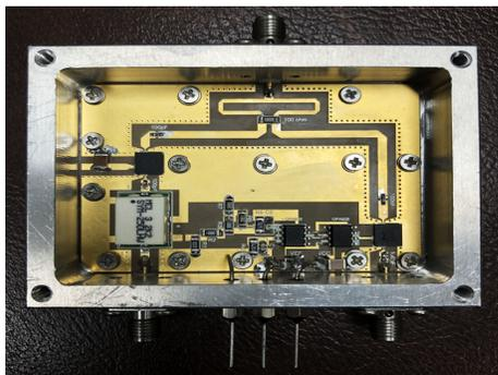
**Fig. 5.** Fabricated PCB of the part of PLL, corresponding to the green box region in Fig.3.
