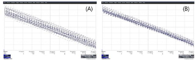
**Fig. 6.** Jittering of magnetron oscillation in case of (A) injection only and (B) PLL over the time span of 1 ns (corresponding to about  $15^\circ$  in phase, where the signals of the magnetron oscillation were down-converted to 41 MHz by a mixer and a precise reference.)
