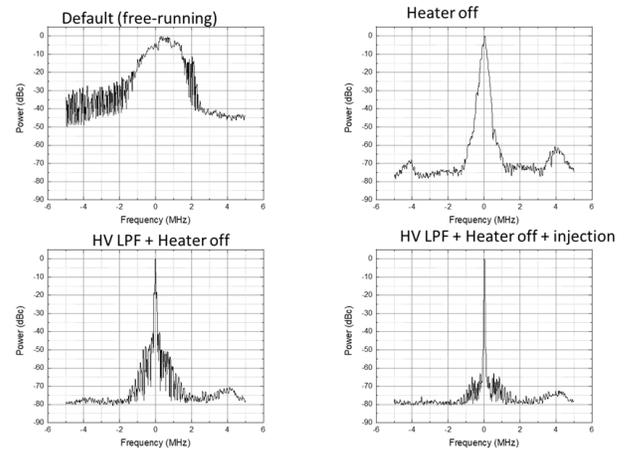
**Fig. 1.** The summary of spectral characteristics of the magnetron in case of default (free-running with heater power), heater-off, employment of high-voltage (HV) low pass filter (LPF) without heater, and injection locking under previous conditions.
