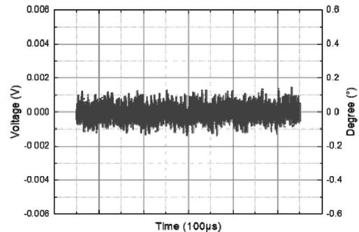
**Fig. 7.** Phase stability (about  $0.3^\circ$  peak-to-peak) of the injection locked magnetron with PLL at the 80% of the maximum power (>800 W) after averaging out thermal noise. Long-term (> 0.5 s) drift of the phase within  $0.24^\circ$  (root-mean-square) was observed, which is exact replication of the anode-voltage variation to maintain the anode-current at a constant value.
