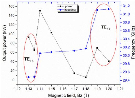
**Figure 3.** The CST simulations results on output power and frequency as the functions of magnetic field, where the beam voltage is 50 kV, beam current is 10 A, pitch factor is 1.3, and the guiding center radius is 8.6 mm.
