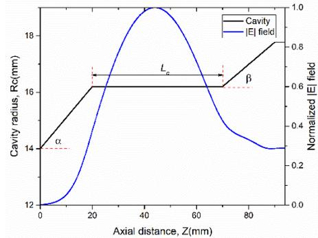
Figure.1. the cold-cavity structure and corresponding cold-cavity normalized electric field profile.
