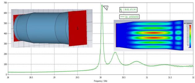
Figure.2. the CST model and the corresponding external quality factor  $Q_e$  of TE<sub>0,3</sub> mode (no.52 in CST), where  $Q_e = \frac{\omega_0 \Gamma_d}{4}$  ( $\Gamma_d$  is the group delay time).
