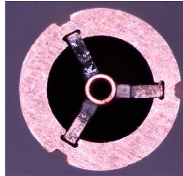
Figure 8. Cross section of the slow wave structure
