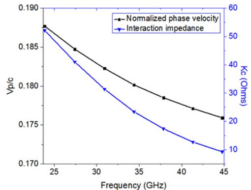
Figure 2. Dispersion and interaction impedance
