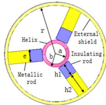
Figure 1. Cross section model of slow wave structure
