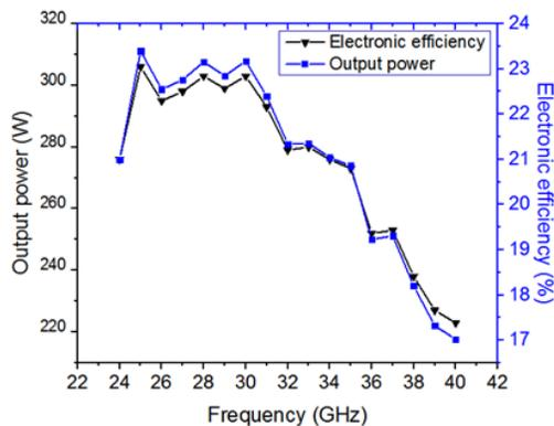
Figure 4. Output power and electronic efficiency versus frequency
