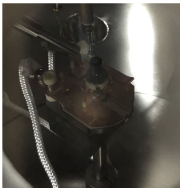
Fig. 1. Single cathode heater inside the Cathode Characterization Chamber.
