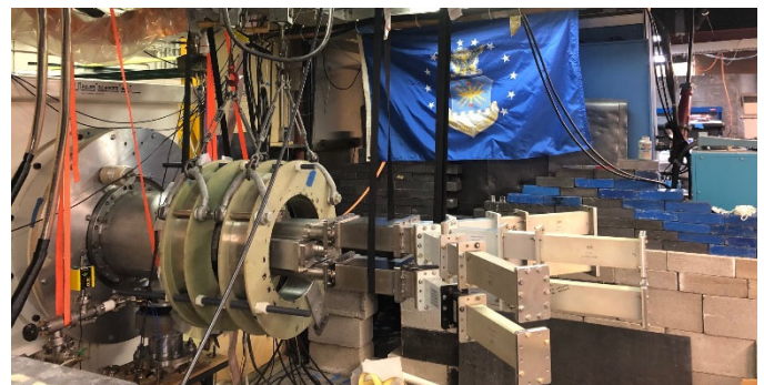
Figure 1: RPM-CACE installed on the MELBA-C driver. Six waveguide directional couplers sample each adjacent pair of the 12 RF cavities.
