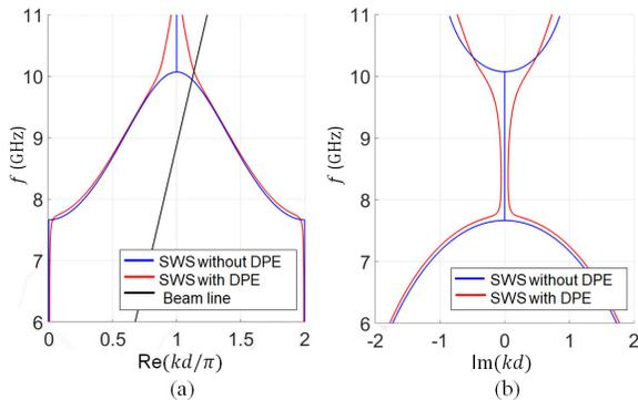
**Fig. 2.** Dispersion of guided modes in the "cold" SWSs in Fig. 1(b) and 1(d), without (blue curve) and with (red curve) distributed power extraction (DPE). (a) Real part and (b) imaginary part of the complex wavenumber. The imaginary part of wavenumber shows that the SWS in Fig. 1(b) exhibits non-zero imaginary part because of the distributed power extraction. The hot SWS with DPE is designed to
