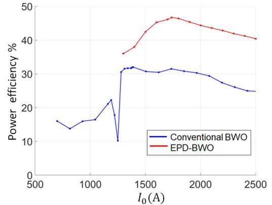
**Fig. 3.** Comparison between the efficiency of a conventional BWO and an EPD-BWO. The EPD-BWO shows improved efficiency at higher level of power generation compared to the conventional BWO.
