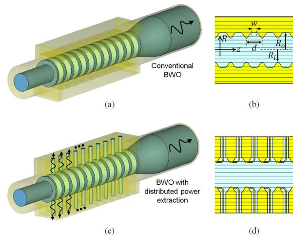
**Fig. 1.** Backward wave oscillator (BWO): (a) conventional BWO where the power is extracted from the waveguide end; (c) EPD-BWO where the power is extracted in a distributed fashion to satisfy the EPD condition [3], [4]. The power is extracted using distributed wire loops (as an example) that are connected to coaxial waveguides as in Ch. 10 in [7]; (b) and (d) are longitudinal cross-sections for SWSs used in both BWOs.
