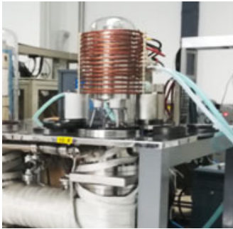
Figure 3. Electron gun degassing
