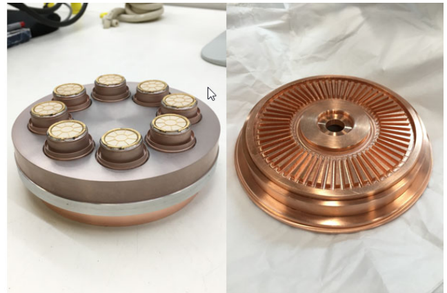
Fig. 4. Multiple beam grid-cathode assembly and coolant side of the anode.
