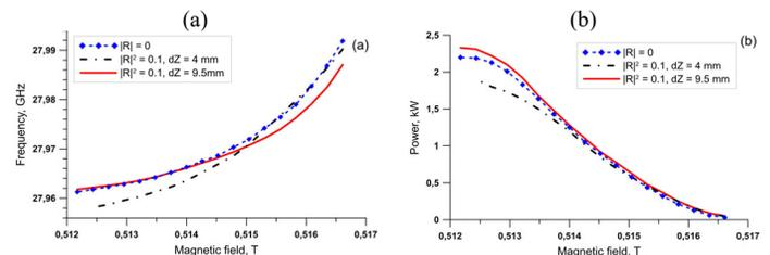
**Fig. 4.** Dependencies of the frequency (a) and power (b) of output radiation on the magnetic field for  $R=0$  (without the reflector).
