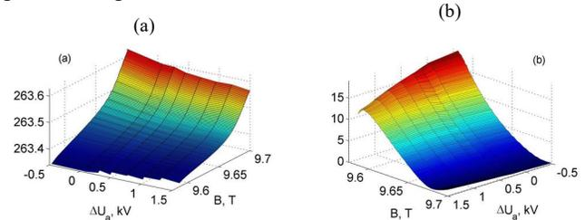
**Fig. 3.** Calculated dependencies of the 263-GHz gyrotron operating frequency (a) and efficiency (b) on the magnetic field and anode voltage.
