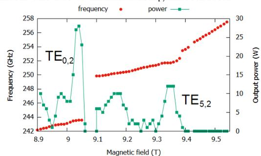
**Fig. 1.** Measured frequency tuning in the 250-GHz gyrotron operating with excitation of low-order  $TE_{5,2}$  and  $TE_{0,2}$  modes.
