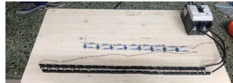
Figure 5. Prototype of the 8-stage Marx generator powered by the 22-stage CW voltage multiplier.
