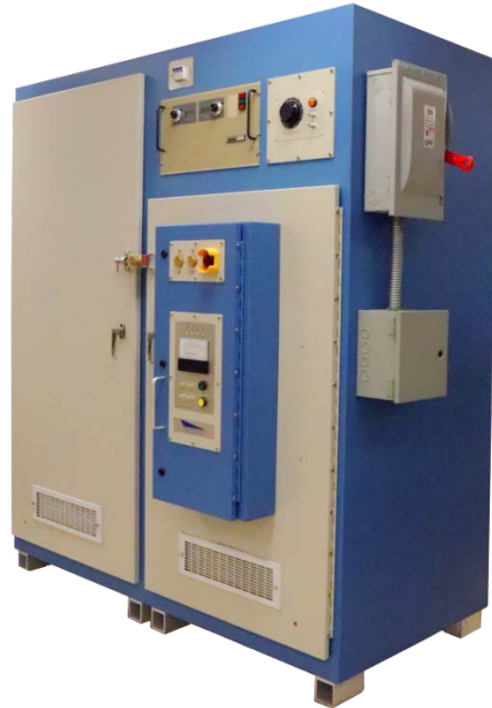
Figure 1. Gyrotron Pulse Modulator Test Stand with HVPS, capacitor bank, filament transformer, and solid-state switch.
