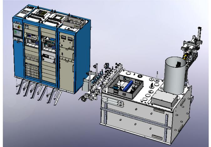
**Figure 1.** C-Band radar transmitter with modulator, klystron tube, RF driver amplifier, waveguide, cooling manifold, HVPS, and control consoles.
