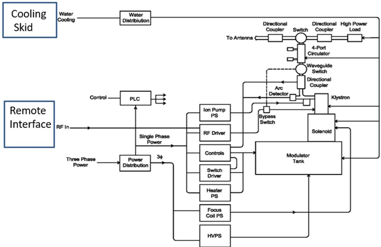
Figure 2. Simplified Transmitter System Block Diagram.
