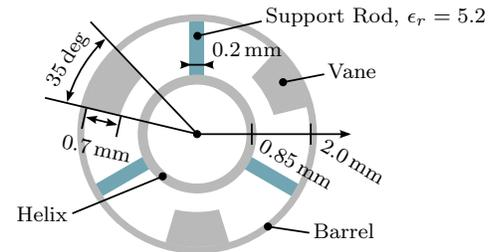
Figure 2. Delay-line cross-section.
