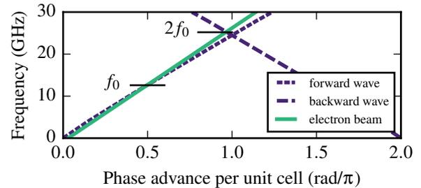
Figure 1. Dispersion of the helix and the beam line.
