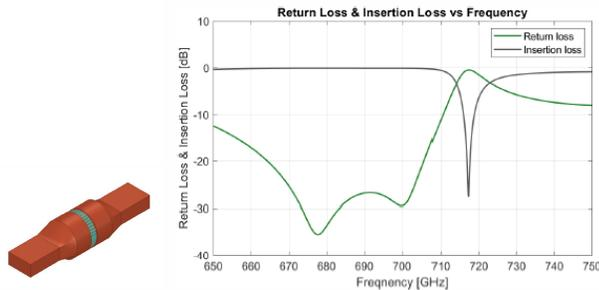
Fig. 5: Left: Solid model of the vacuum window, Right: Transmission properties of the window.
