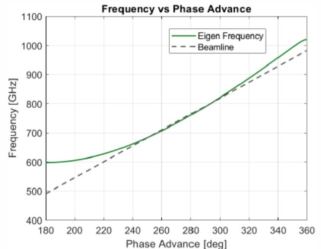
**Fig. 2: Dispersion diagram of the circuit.**
