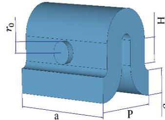
**Fig. 1: Key dimensional parameters of the circuit.**
