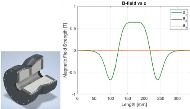
Fig. 4: Left: Solid model of the magnet system for the TWT and Right: On-axis field profile.
