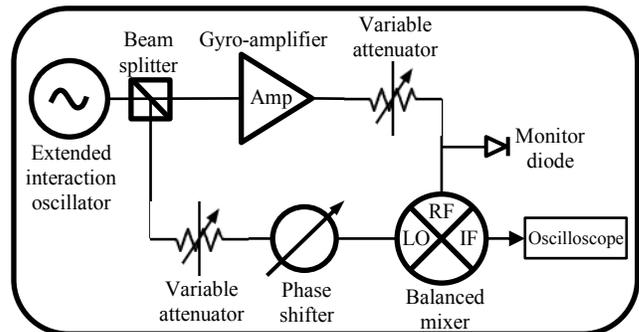
**Figure 1.** Schematic of the diagnostic setup for phase shift and phase stability measurements.
