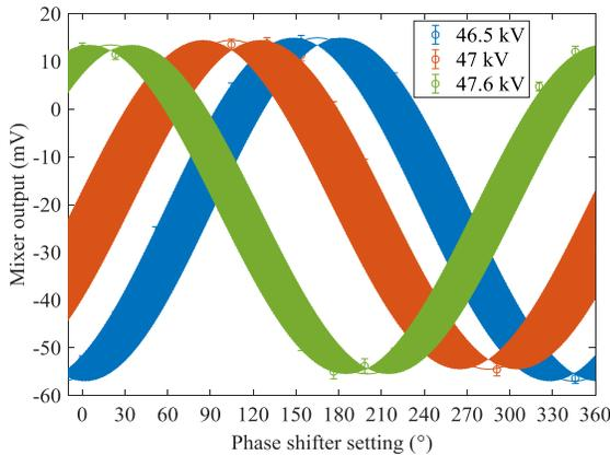
**Figure 2.** Mixer DC output as a function of phase shifter setting measured at three cathode voltages. The smooth curves show sine waves fitted to the data, with the uncertainties in the fit represented by the shades areas.
