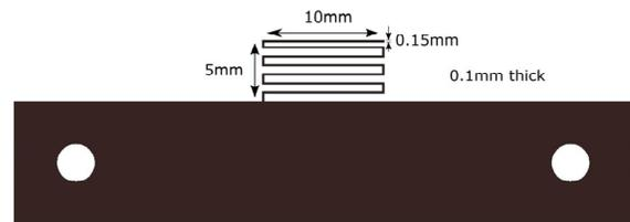
**Figure 1.** Cross-section of single period of meandered-wire metamaterial with dimensions used in experimental prototype. The bottom portion with holes is used for mounting and construction.
