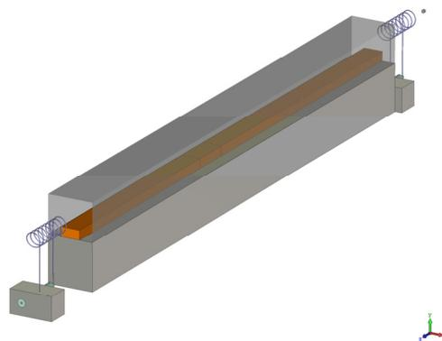
**Figure 2.** A CAD diagram of the experimental prototype with the MTM visualized using a rectangular bulk medium. The MTM is placed inside a cutoff rectangular waveguide. Input and output helices are positioned on either side to couple power into and out of the structure.
